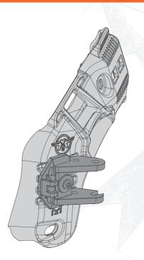
6 Reinstall center screw. Torque 16-18 in-lb. When properly tightened, AMP™ Helmet Adapter Arm assembly will funtion as it would on Ops-Core™ ARC™ Rail.
