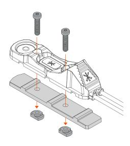
Place the AXON™ XL Control Module on the M-LOK® Rail in desired location. Ensure the M-LOK® nuts are fully perpendicular to the M-LOK® slot in rail (fully seated).
