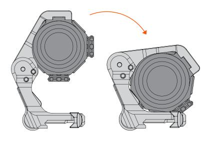
Bring the magnifier into the up position. From the inside of the base, depress the safety on the interior of the integrated FAST<sup>TM</sup> QD Lever. Push outward and the QD Lever will open fully. The QD Lever may need to be held flush with the mount base while depressing the safety.
