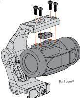
The FAST™ FTC OMNI mount uses a force-to-overcome mechanism. Grasp the magnifier body and pivot assembly down to the stowed position. Repeat in reverse to bring the magnifier back into the active position.
