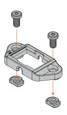
Guide the ModButton™ Lite Control Module through open slot of M-LOK® Mounting Kit until fully seated.
