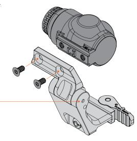
The FAST™ FTC PA mount uses a force-to-overcome mechanism. Grasp the magnifier body and pivot assembly down to the stowed position. Repeat in reverse to bring the magnifier back into the active position.
