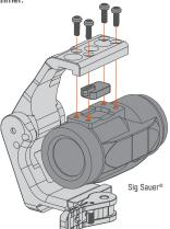
The FAST™ FTC OMNI mount uses a force-to-overcome mechanism. Grasp the magnifier body and pivot assembly down to the stowed position. Repeat in reverse to bring the magnifier back into the active position.
