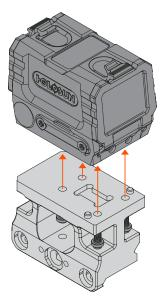
Insert each Clamp Screw through a Washer. Then insert them through the FAST™ AEMS mount and thread them into the Rail Clamp. Secure screws using a T25 bit driver. Lightly snug all screws before applying final torque to any. **Torque to 35** in-Ibs (4 Nm).
